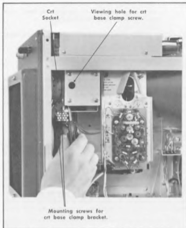
Fig. 4-3. Loosening the crt base clamp.
