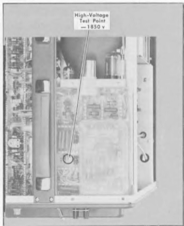
Fig. 5-3. High-voltage test point location.
